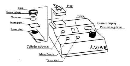
Figure 1. The gravimetric water retention meter
